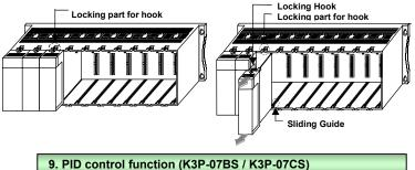
K3P-07BS and K3P-07CS module include PID (Proportional Integral Differential) function, and no external PID module is required.
